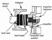
Figure 1 - Mechanical Seal Replacement for Threaded Shaft (379 Series).
