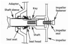
Figure 2 - Mechanical Seal Replacement for Keyed Shaft (365 Series).
